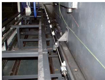
An installation of 7600mm long of 19F for 6600 ton two plated plastic injection machine.
