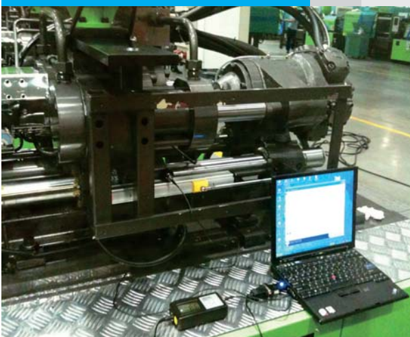
On-site shock and vibration test
