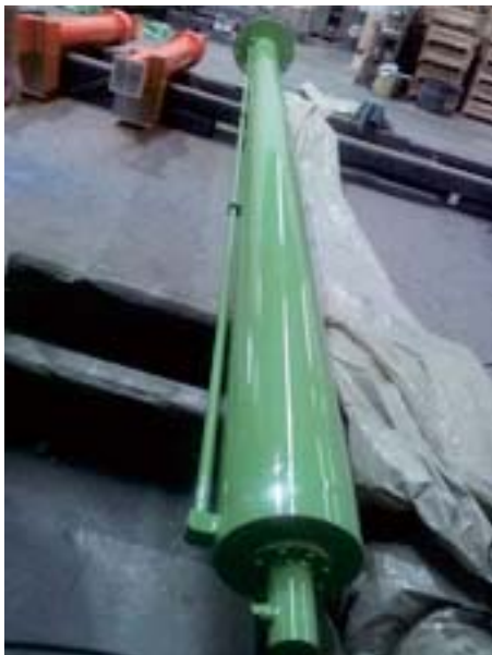
6550mm hydraulic cylinder uses 19 series
