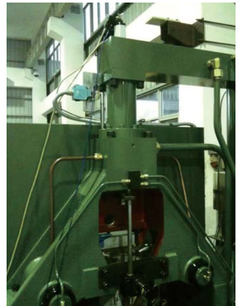
Hot chamber die-cast machine used Germanjet 17 series
